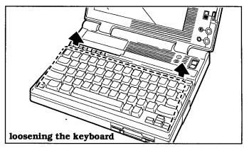
6. Raise the rear of the keyboard several inches, rotate the rear of the keyboard 180 degrees toward you, and place the keyboard in front of you with the keys facing down as shown in the following figure.
